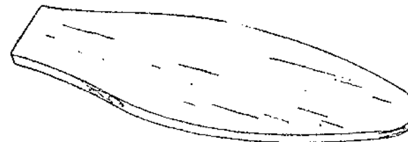
Cement airscrew blades securely to hub.
